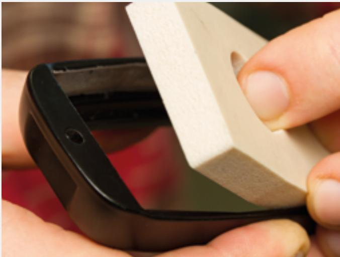
Masking with grip cut in silicone rubber foam DSS
