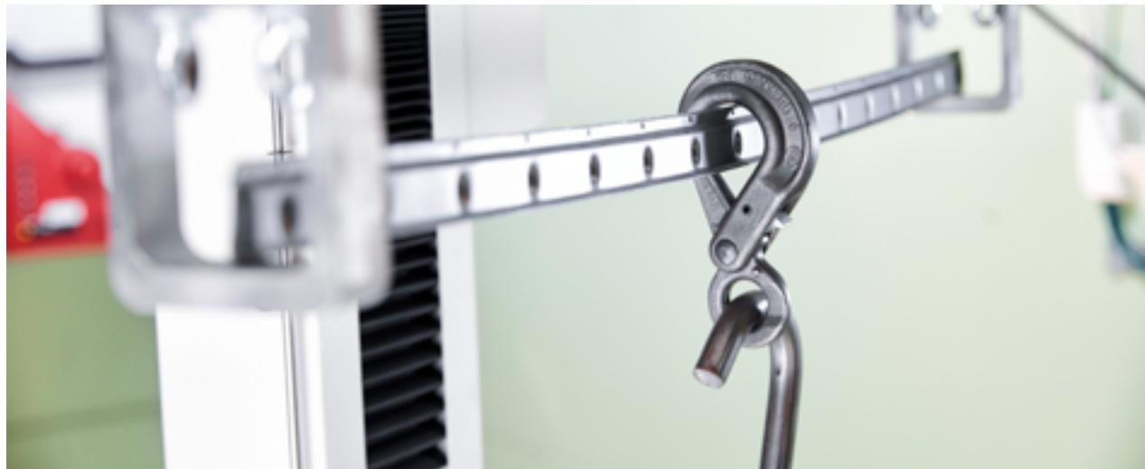
Pull test of suspension beam.
