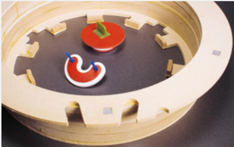
Glued rubber sheets in solid DSG and foamed silicone DSS with grip and glued MDF maskings with magnets
